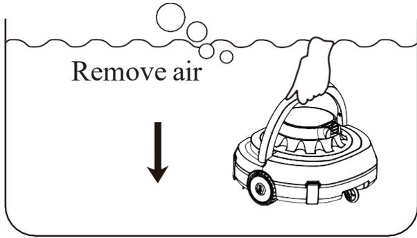
1. Press the on/off button located under the cleaner until the button lights up. Hold the robot horizontally under the water for approximately 20-30 seconds. The robot should sink freely down to the bottom of the pool.
