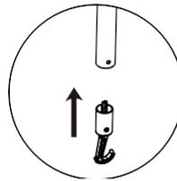
3. If the water is deep, the robot can be hooked up with a hook.
