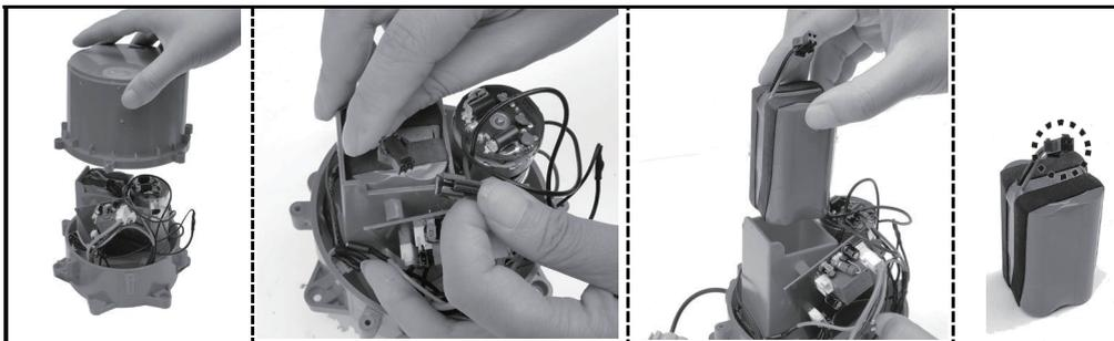
3. Open the battery cover, find the battery connection line, press the clip on the connector, pull it out, and take out the battery.
