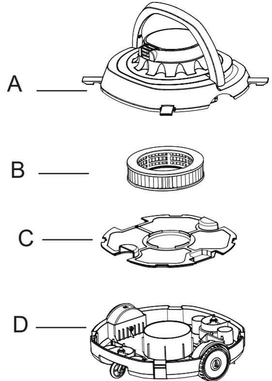
The jet head (A) rotates 180 degrees as the water flows through the bottom base (D), the filters (C & B) and the upper cover (A). The water flow passing through the jet head propels the robot across the pool floor. Should an obstacle prevent the robot from moving forward, the jet head turns 180 degrees and sends the robot in the opposite direction. Large debris is collected and stored in the bottom base (D) of the cleaner while fine debris is trapped by the filter (C),
